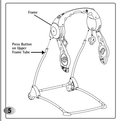
• Insert the upper frame tubes into the frame until you hear a "click" on both sides.
